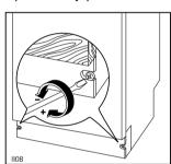
Fitting the decor panel may sometimes affect this balance. In this case it will be necessary to adjust the balance as follows:
